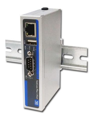
DSK-NCP: Side-mount on DIN-Rail >Back
